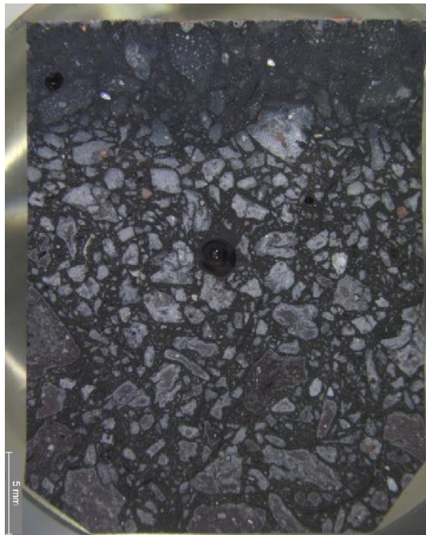
Fig.1 DSF CTB Core Section, no visible delamination plane between dark and light layers. Core sample taken from block ~9 years into campaign; block was available due to power outage and bath loss.
